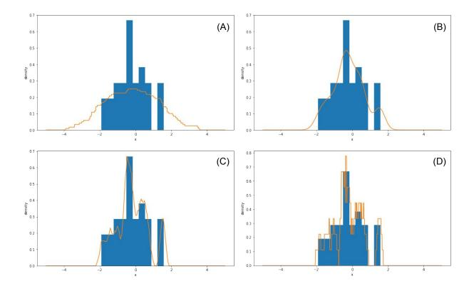
**Solution:** (A) and (D) are the boxcar kernel since there are visible "square" edges. Gaussian kernel would yield smooth edges and the triangular kernel would yield triangular edges.
